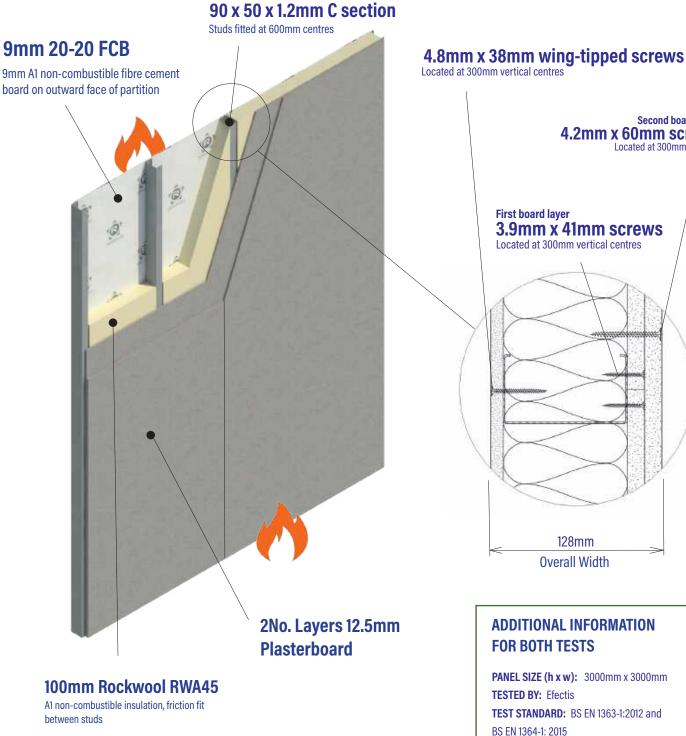
Second board layer 4.2mm x 60mm screws Located at 300mm centres
