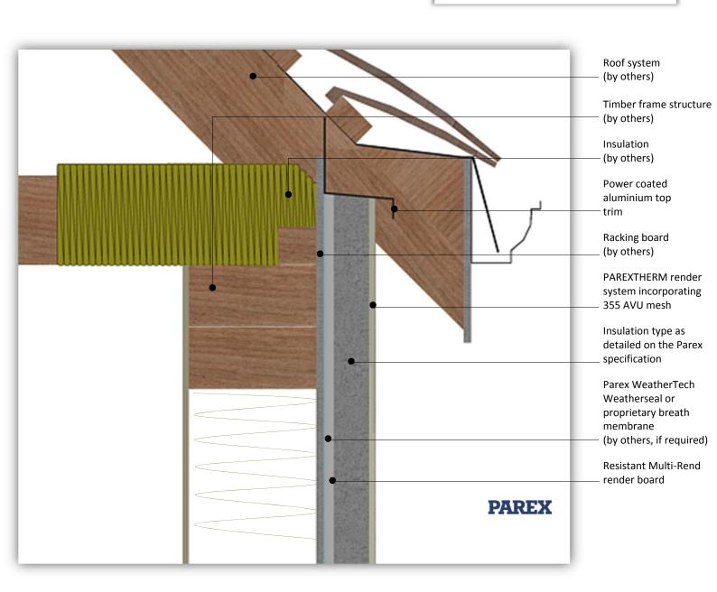
System: PAREXTHERM onto Timber Frame
