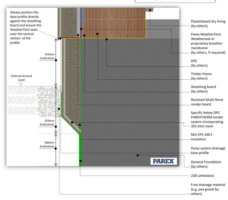
System: PAREXTHERM onto Timber Frame
