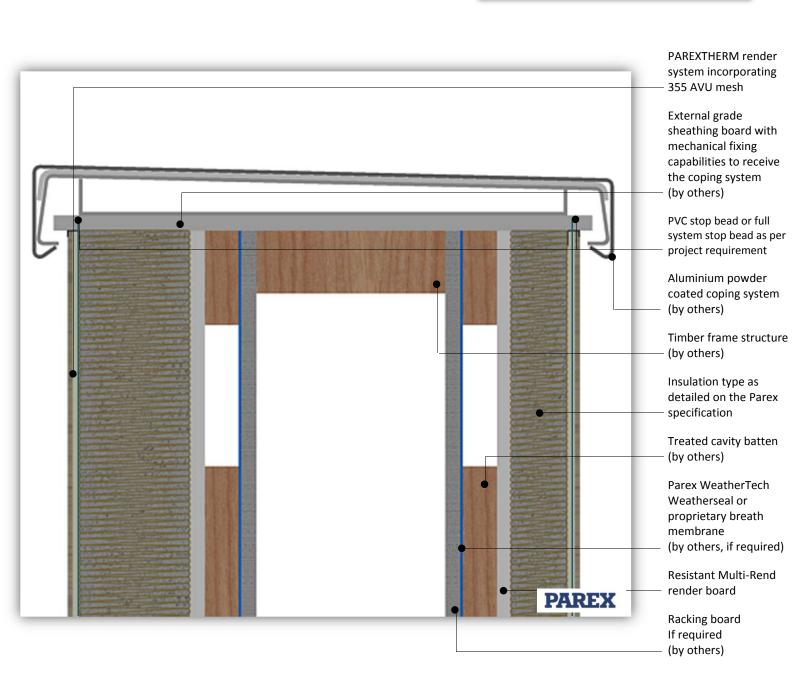
System: PAREXTHERM onto Timber Frame
