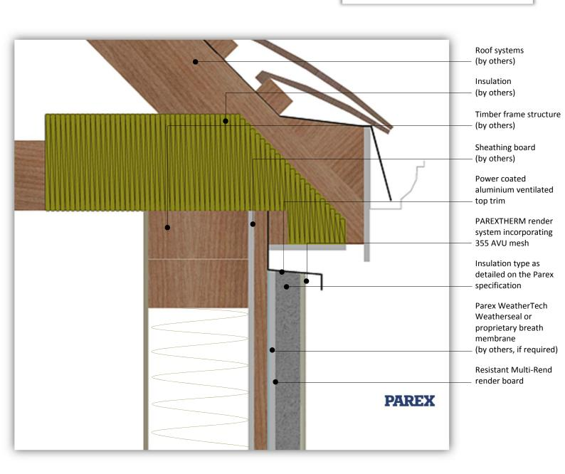
System: PAREXTHERM onto Timber Frame
