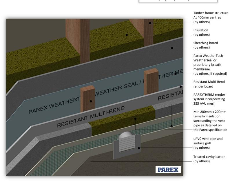
System: PAREXTHERM onto Timber Frame
