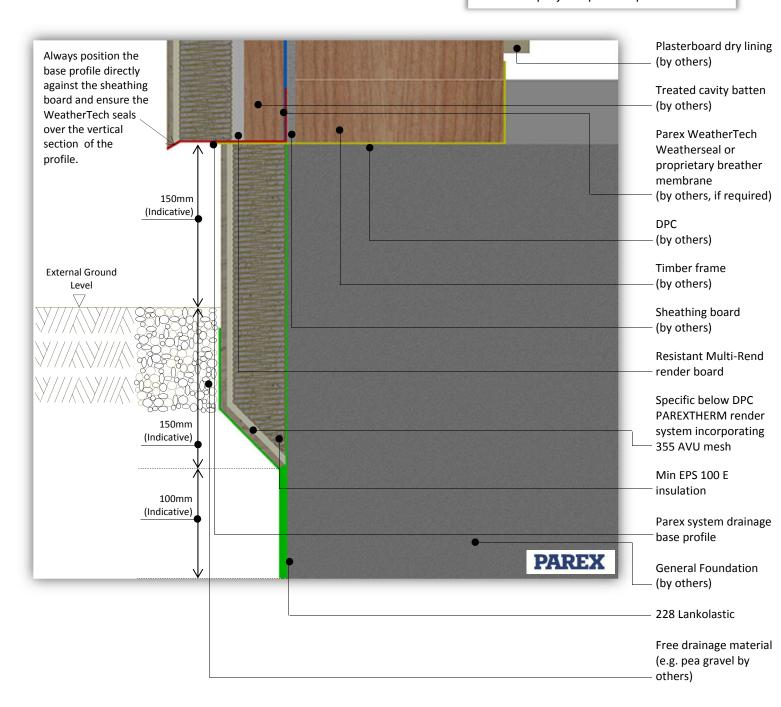
System: PAREXTHERM onto Timber Frame
