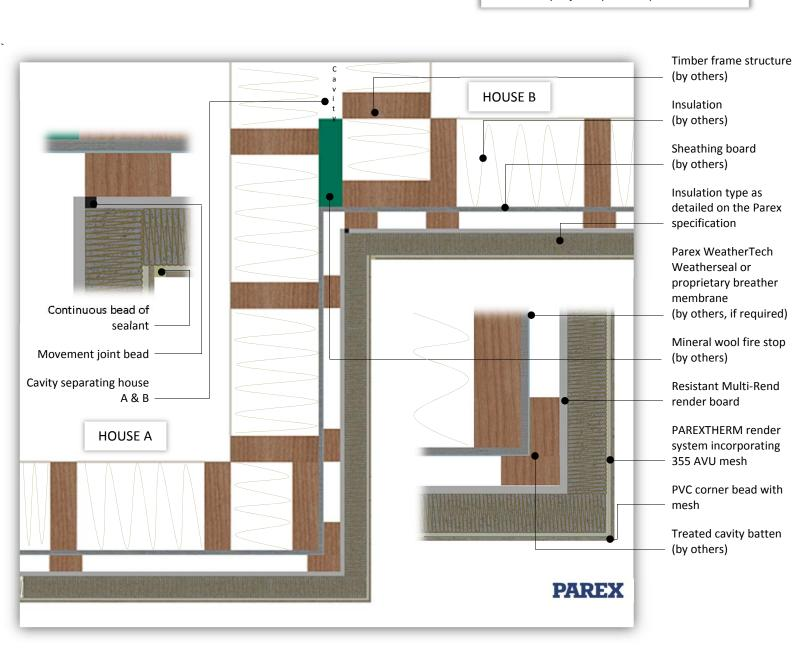
System: PAREXTHERM onto Timber Frame
