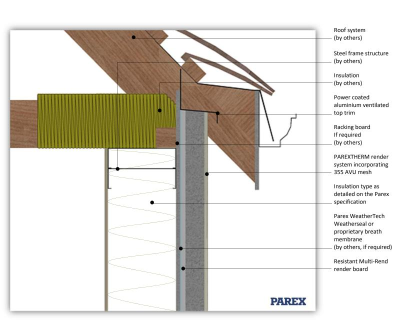
System: PAREXTHERM onto Steel Frame
