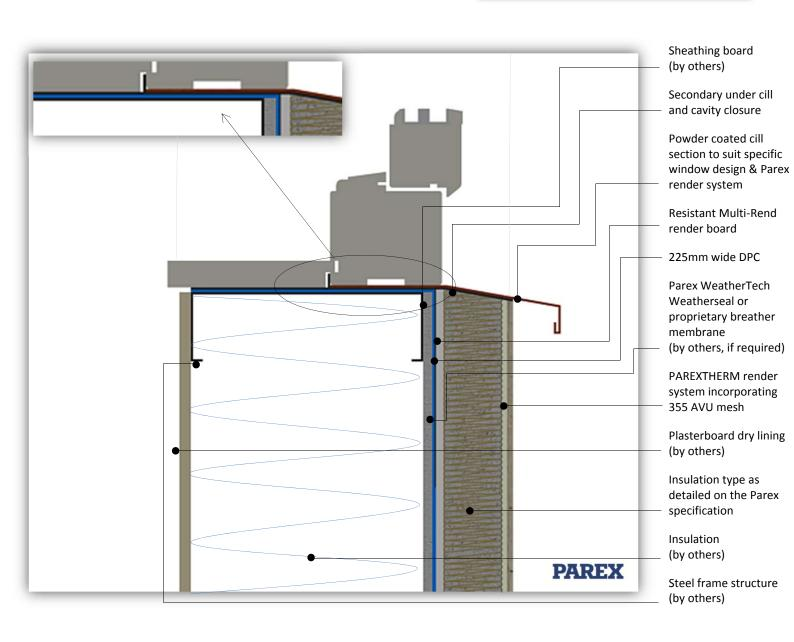
System: PAREXTHERM onto Steel Frame
