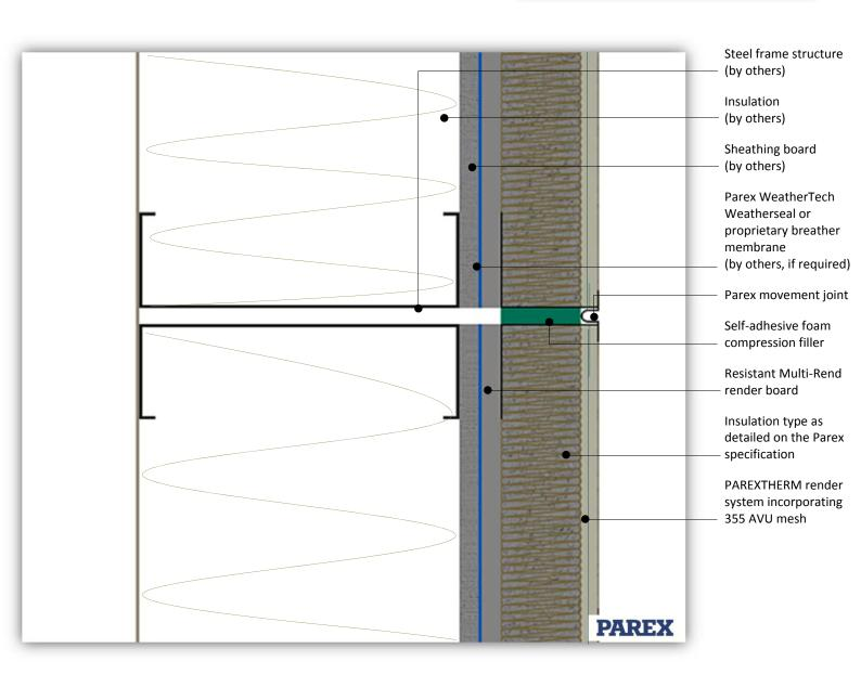
System: PAREXTHERM onto Steel Frame
