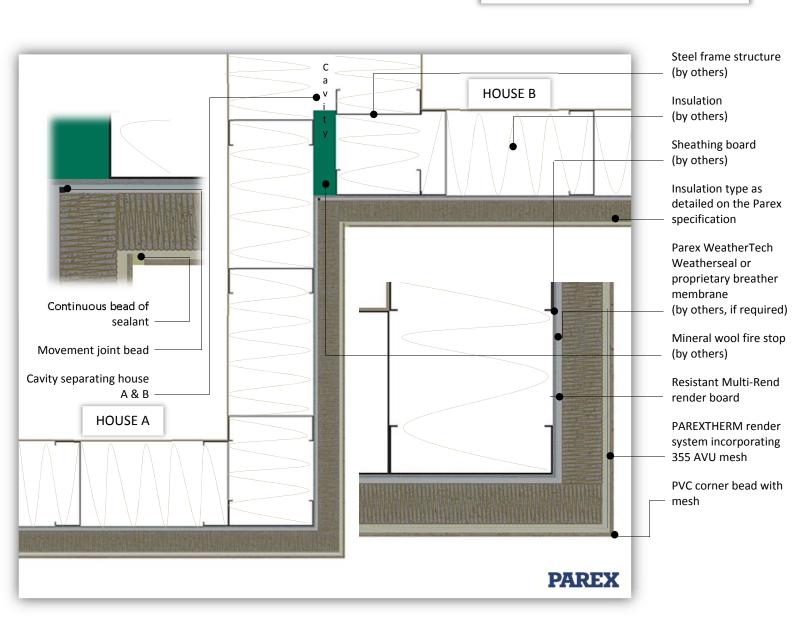
System: PAREXTHERM onto Steel Frame
