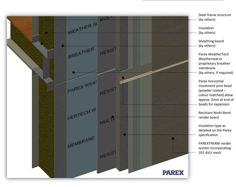
System: PAREXTHERM onto Steel Frame
