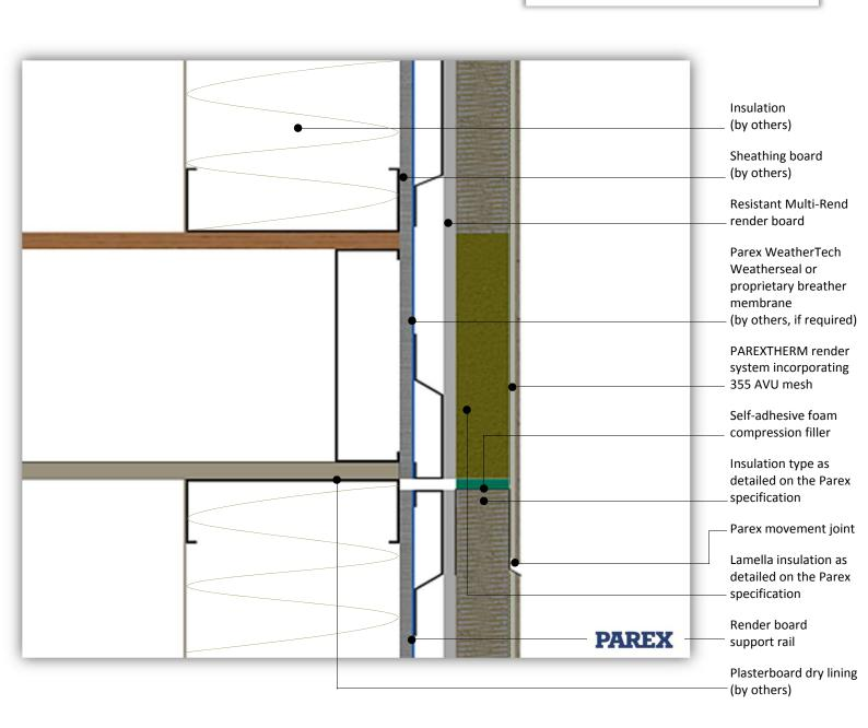
System: PAREXTHERM onto Steel Frame
