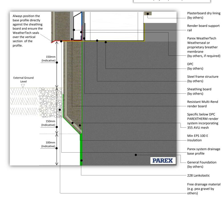
System: PAREXTHERM onto Steel Frame
