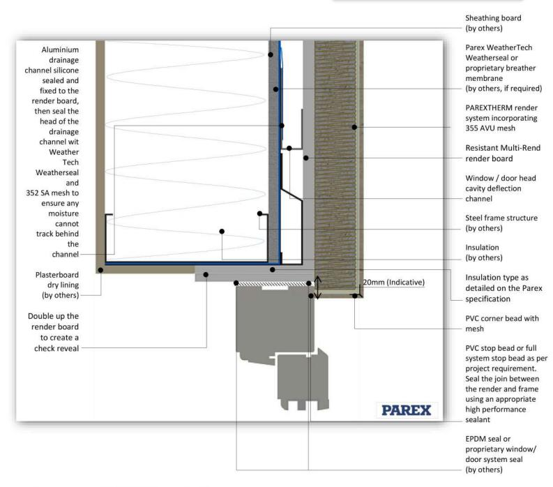
System: PAREXTHERM onto Steel Frame
