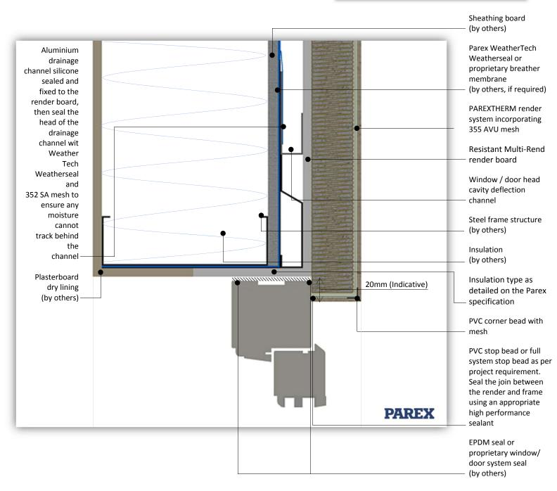
System: PAREXTHERM onto Steel Frame
