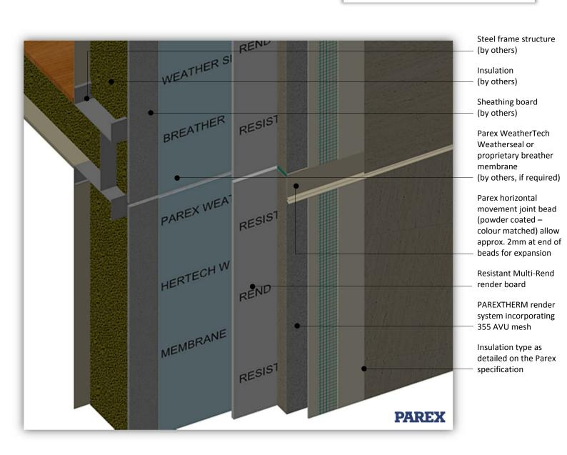
System: PAREXTHERM onto Steel Frame
