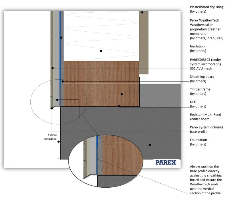
System: PAREXDIRECT onto Timber Frame
