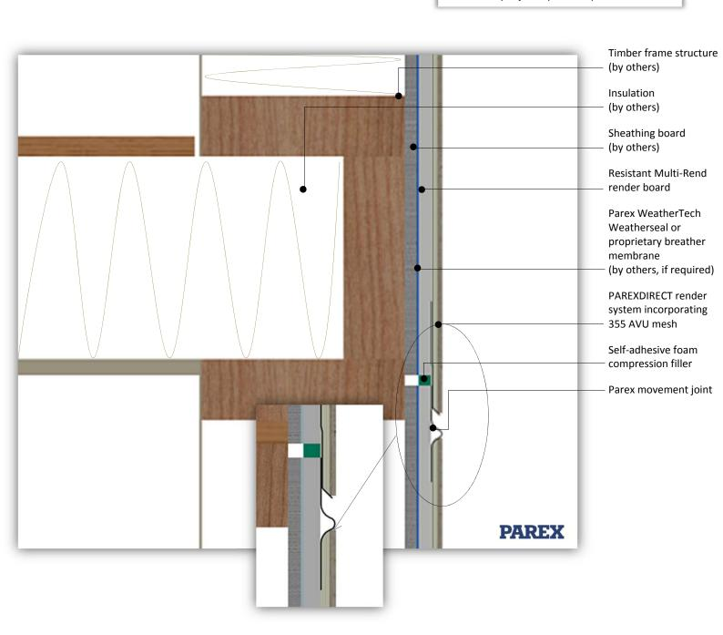
System: PAREXDIRECT onto Timber Frame
