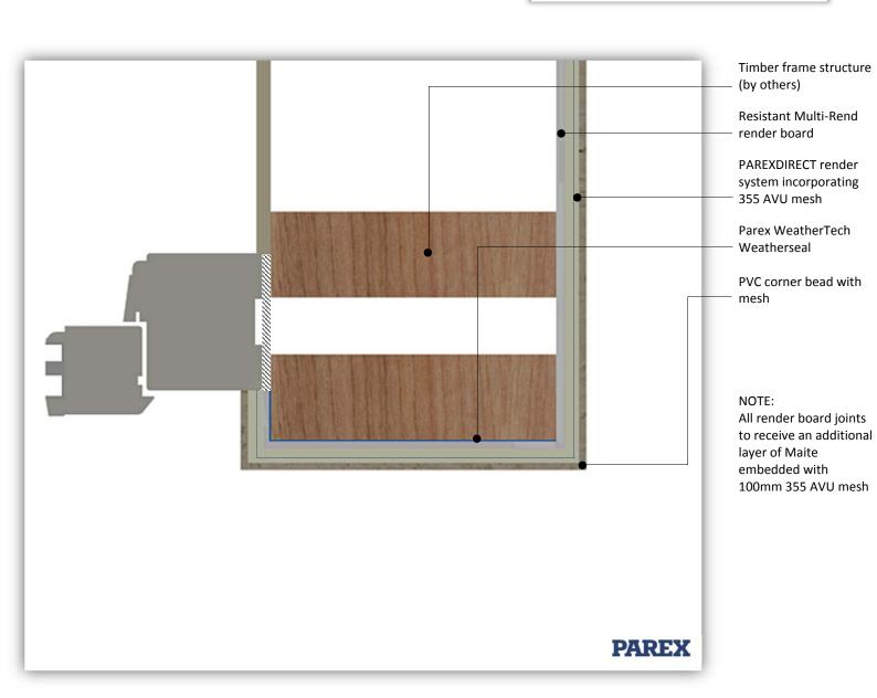
System: PAREXDIRECT onto Timber Frame
