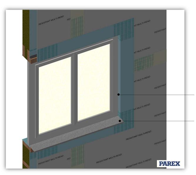
Fully seal the window with an appropriate mastic or silicone sealant to ensure the frame is fully weatherproof against water ingress
