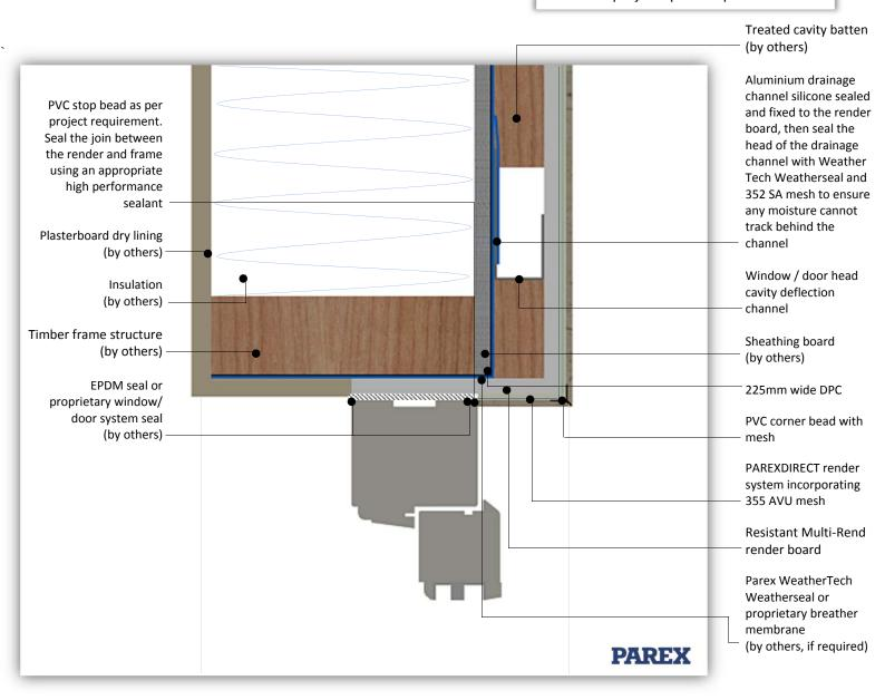
System: PAREXDIRECT onto Timber Frame
