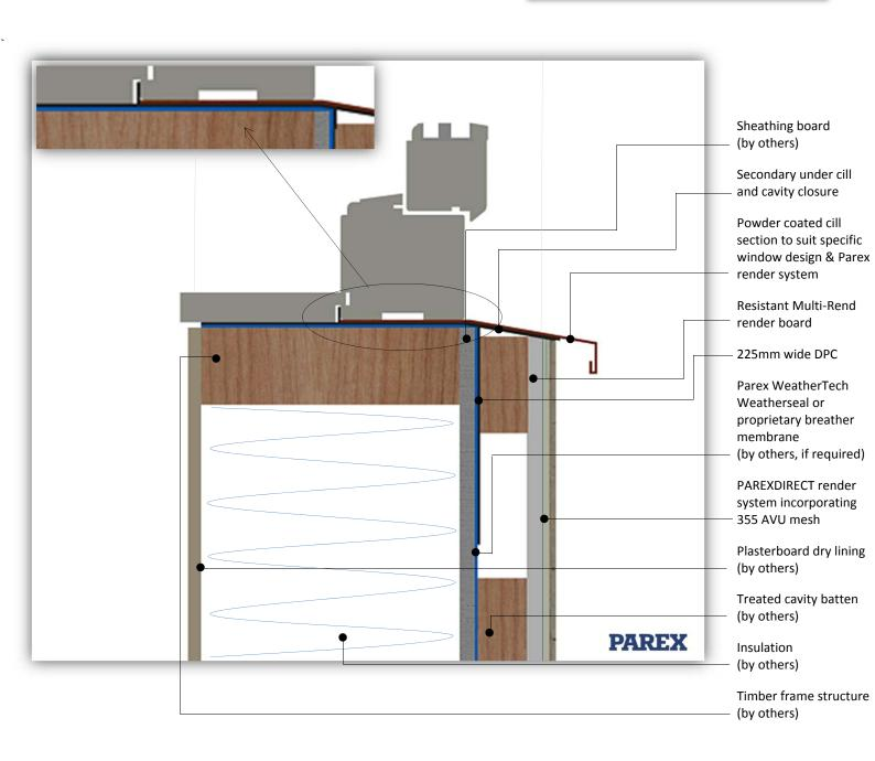
System: PAREXDIRECT onto Timber Frame
