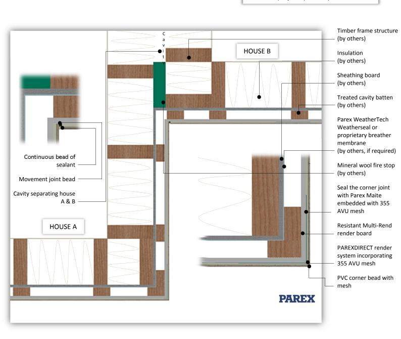
System: PAREXDIRECT onto Timber Frame
