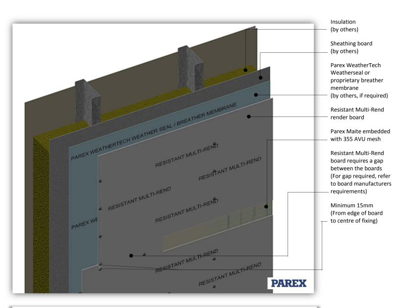
To ensure you meet with project specific requirements, consult the Resistant Multi-Rend render board fixing requirements. All fixings to be Resistant Multi-Rend non-corrosive and of sufficient length and performance. The fixing distances shown are for guidance only and may vary subject to the building design. If you are unsure please ask first.
