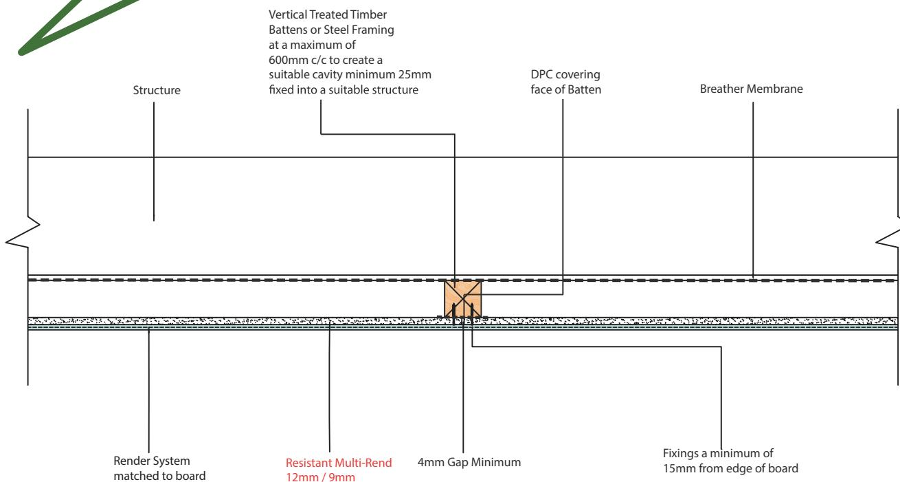
**\*Multi-Rend board must be dry, clean & free from dust etc before a render is applied to the board\***
