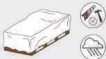
sheets will cause permanent surface staining. They should be protected from the weather and other trades on site at all times.
