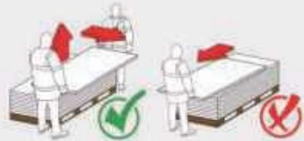
Boards should always be lifted by two people and not dragged across each other to prevent unnecessary scratching or damage.
