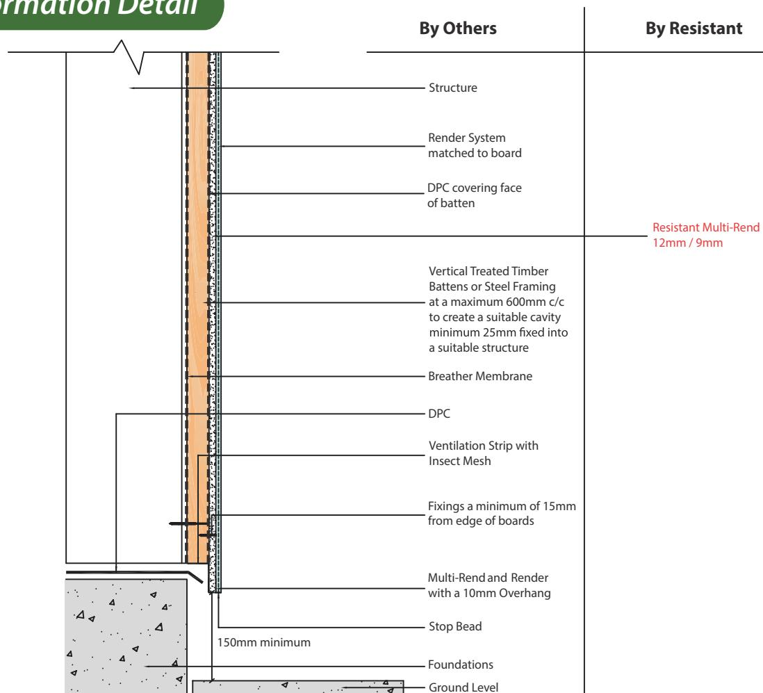
\*Multi-Rend board must be dry, clean & free from dust etc before a render is applied to the board\*
