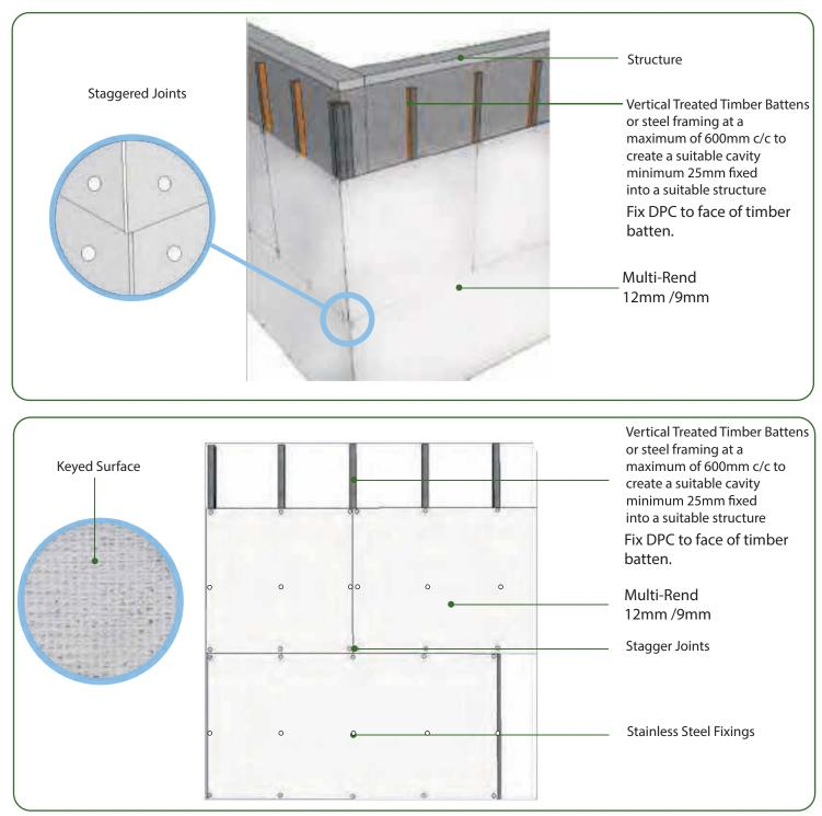
\*Multi-Rend boards must be fitted horizontally to create a brick bond effect. This will stagger joints and increase the strength of the overall boards. If fixed at 300mm centres 27 fixings per board will be required.\*
