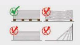
from the ground on a pallet, in dry conditions indoors and be under cover. Boards should not be leant upright for long periods of time.
