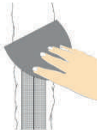
7. Bed scrim cloth over all joints (both walls & floors) using the tile adhesive to provide extra reinforcement.
