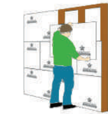
4. Offset boards when fixing. Four corners should never meet. The tiling side (coarse side) is marked on all boards.
