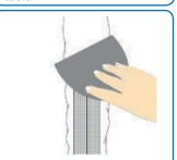
7. Bed scrim cloth over all joints (both walls & floors) using the tile adhesive to provide extra reinforcement.
