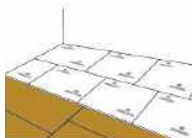
5. Check the subfloor is free from debris and completely flat. Minor differences in levels can be evened out by spreading a thin layer of tile adhesive on to the subfloor. Fix the 6mm Multi-pro Tile Backer board to the floor at 200mm fixing centres using countersunk screws.
