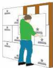
4. Offset boards when fixing. Four corners should never meet. The tiling side (coarse side) is marked on all boards.
