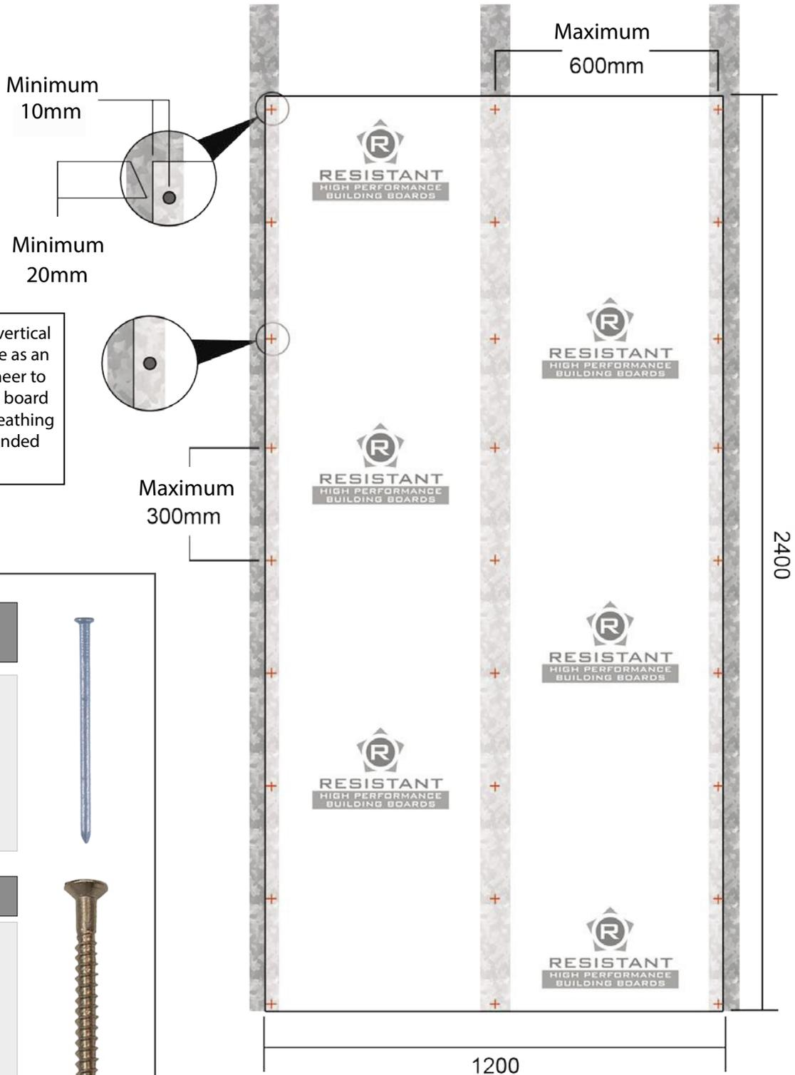
Please note guidance stated for vertical fixing centres is maximum for use as an internal wall lining. Project engineer to specify fixing distances for when board is used as a structural racking sheathing board or as a component of a bonded cladding panel.
